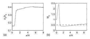
FIG. 21.  $\tau$ =0.41, case R6. (a) Computed mean pressure along the (—) upper and (— —) lower wall. (b) Computed mean Mach number along the center line y=0, (— —) theoretical value downstream the shock provided by Eq. (1).
