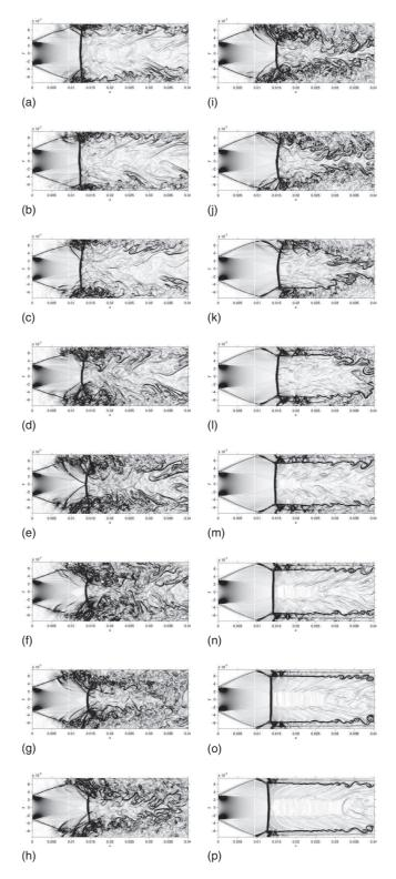
FIG. 22. Pressure ratio  $\tau$ =0.41, case R6. Schlieren pictures  $|\nabla \rho|$  around the nozzle exit in the middle x-y plane. Snapshots over a period of the self-excited base-pressure oscillations.
