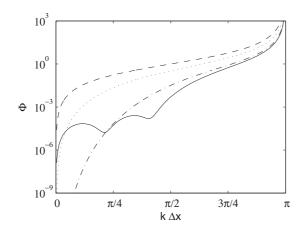
FIG. 24. Transfer function of the detector strength  $\hat{\Phi}_i^{\xi}$  given by Eq. (A2) as a function of the normalized wavenumber  $k\Delta x$ . (---) Second-order filter (classical Jameson, n=1);  $(\cdots\cdots)$  fifth-order filter (n=2);  $(-\cdots-)$  tenth-order filter (n=5); (---) 11-point optimized filter (n=5).
