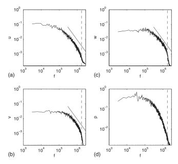
FIG. 12. Pressure ratio  $\tau$ =0.15, case R1. Frequency spectra at (x,y) =  $(3.5H, 15\Delta y^+)$  for the three velocity components and for the pressure. The dashed line designates the cutoff frequency of the algorithm, estimated using Taylor's hypothesis, and the solid line represents Kolmogorov's 5/3-law.
