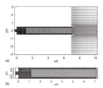
FIG. 4. Grid generated by using ogen for case R1 corresponding to a pressure ratio  $\tau$ =0.15; see Table I. Every eighth line is represented in the *x-y* plane. (a) Entire computational domain including the nozzle, the expansion duct, and the plenum chamber. (b) Detailed view on the nozzle and of the expansion duct. The walls are refined using overlapping grids.
