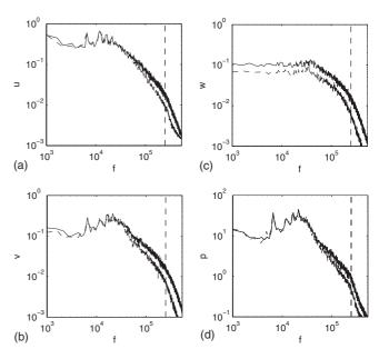
FIG. 18. Pressure ratio  $\tau$ =0.32, case R4. Frequency spectra at (x,y) =  $(3.5H, 15\Delta y^+)$  for the velocity components and for the pressure, using (---) the Jameson sensor and (--) the modified Jameson sensor based on 11-point selective filter. The vertical dashed line designates the cutoff frequency of the algorithm, estimated by using Taylor's hypothesis.
