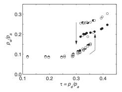
FIG. 2. Turbulent flow behind a sudden enlargement of rectangular duct cross section for the case  $L=0.16\,$  m, L/H=4.82, and h/H=0.3. Experimental data (Ref. 2) of the ( $\bigcirc$ ) upper and ( $\bigcirc$ ) lower normalized mean base pressure  $p_w/p_a$  as a function of the pressure ratio  $\tau$ .
