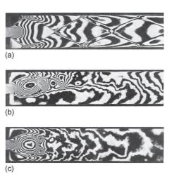
FIG. 3. Mach–Zehnder interferometry visualizations of the flow, i.e., fringes represent lines of constant density, for different pressure ratios: (a)  $\tau$  = 0.151 symmetrical supersonic flow, denoted regime A; (b)  $\tau$ =0.364 symmetrical flow with a normal shock, denoted regime B; (c)  $\tau$ =0.377 asymmetrical flow with jetlike shock cells, denoted regime C. The expansion duct length is L=0.24 m and the aspect ratios are L/H=7.23 and h/H=0.3, taken from Ref. 3.
