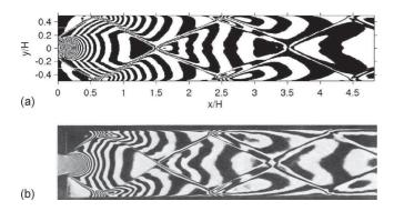
FIG. 6. Pressure ratio  $\tau$ =0.15, case R1. Mean density field using interferogram-like color map. (a) Present computation, 60 isocontours between 0 and 0.742 kg m<sup>-3</sup>; (b) experiments (Ref. 3).
