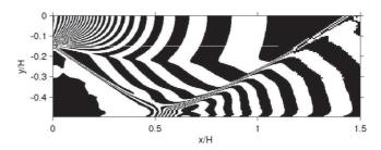
FIG. 7. Pressure ratio  $\tau$ =0.15, case R1. Zoom on the reattachment zone of the abruptly expanded supersonic jet; refer to Fig. 6.
