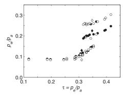
FIG. 13. Experimental data (Ref. 3) of the normalized mean base pressure  $p_w/p_a$  as a function of the pressure ratio  $\tau$  for cases R2–R5, see also Fig. 2, and the present simulations:  $(\diamondsuit)$  upper wall and  $(\spadesuit)$  lower wall.
