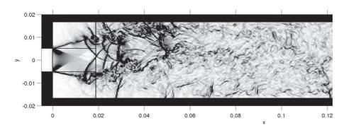
FIG. 16. Pressure ratio  $\tau$ =0.32, case R4. Schlieren-like view  $0 \le |\nabla \rho| \le 200$  kg m<sup>-4</sup> of the main channel on the middle *x*-*y* plane.
