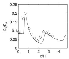
FIG. 8.  $\tau$ =0.15, case R1. Static mean pressure distribution along the duct wall and normalized by  $p_a$ ; (—) present computation; ( $\bigcirc$ ) experiments (Ref. 3).
