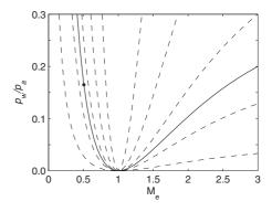
FIG. 26. Curves  $p_w = p_w(M_e)$  for  $\phi = 0.1, 0.3, 0.5, 0.7, 0.9$  in dashed lines. Solid curve for  $\phi = 0.4$  corresponding to case R6 ( $\bullet$ )  $p_w/p_a \approx 0.165$  and  $M_e \approx 0.51$ .
