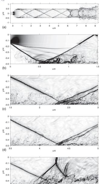
FIG. 9. Pressure ratio  $\tau$ =0.15, case R1. Instantaneous numerical Schlieren field,  $0 \le |\nabla \rho| \le 60\,$  kg m<sup>-4</sup>. (a) Entire computational domain; (b) jet reattachment region; (c) first shock wave/boundary layer interaction zone; (d) second shock wave/boundary layer interaction zone; (e) third shock wave/boundary layer interaction zone with flow separation near the end of the duct, at x/H=7.23.
