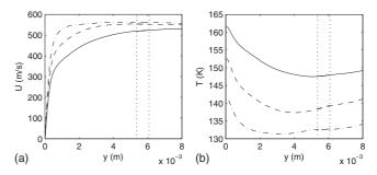
FIG. 10. Pressure ratio  $\tau$ =0.15, case R1. Profiles of the mean streamwise velocity U (a) and temperature T (b) at three different positions: (----·)  $x_{P_1}$ =1.5H, (- - -)  $x_{P_2}$ =3.5H, and (—)  $x_{P_3}$ =5.5H. Dotted lines denote the overlap region.
