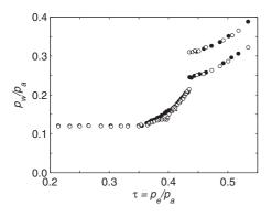
FIG. 19.  $\tau$ =0.41, case R6. Normalized mean base pressure measured (Ref. 3) as a function of the pressure ratio  $\tau$ , ( $\bigcirc$ ) upper wall and ( $\blacksquare$ ) lower wall. Present simulations, ( $\square$ ) upper wall and ( $\times$ ) lower wall.
