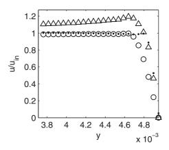
FIG. 5. Velocity profiles of the incoming laminar boundary layer at three locations: ( $\bullet$ ) at  $x=-L_n$ , ( $\bigcirc$ ) at  $x=-L_n/2$ , and ( $\triangle$ ) at x=0, where  $L_n=9.1\times 10^{-3}$  m is the nozzle length.
