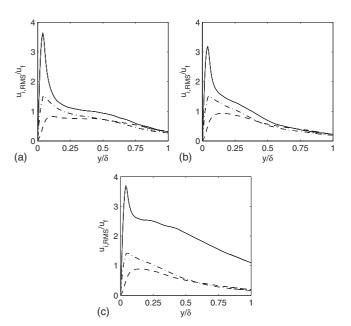
FIG. 11. Pressure ratio  $\tau$ =0.15, case R1. Transverse profiles of (—) u', (- - -) v', and (-····) w' at three different positions: (a)  $x_{P_1}$ =1.5H, (b)  $x_{P_2}$ =3.5H, and (c)  $x_{P_3}$ =5.5H.
