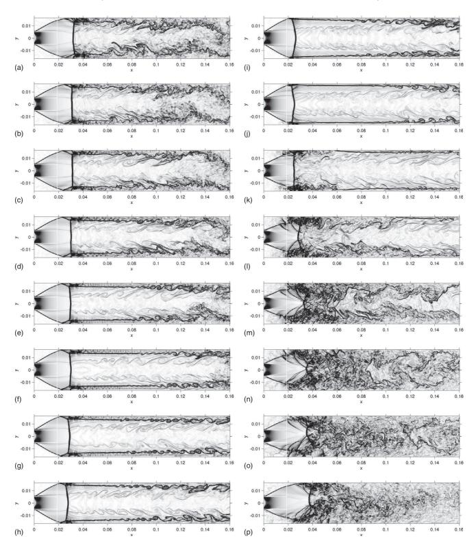
FIG. 15. Pressure ratio  $\tau$ =0.31, case R3. Schlieren-like pictures  $0 \le |\nabla \rho| \le 80\,\text{ kg m}^{-4}$  of the whole channel duct in the middle *x-y* plane. Snapshots over a period of the base-pressure oscillations.
