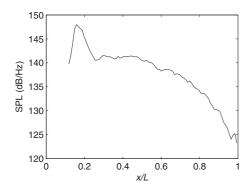
FIG. 23. Pressure ratio  $\tau$ =0.41, case R6. Computed sound pressure level of the wall pressure along the main channel for the frequency peak at f $\simeq$  700 Hz with a spectral resolution  $\Delta f$ =50 Hz.
