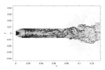
FIG. 20. Schlieren-like view  $0 \le |\nabla \rho| \le 80$  kg m<sup>-4</sup> in the middle *x-y* plane of the whole computational domain including the reservoir.
