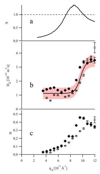
FIG. 4. a) Static structure factor  $S(q_{\perp})$ . b) Diffusion coefficient  $D_{N,\perp}(q_{\perp})$ . The symbols correspond to two different measurements performed on the same sample. The solid line and the greyed area are the fit by a sigmoidal function and the  $\pm \sigma$  prediction bands (see text). c) Hydrodynamic function obtained using Equation 2. The data are plotted against a common  $q_{\perp}$  axis.
