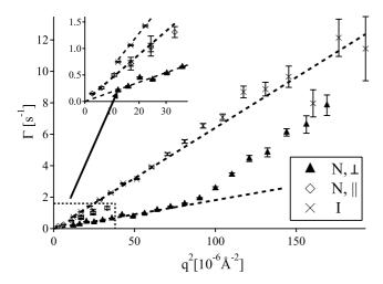
FIG. 3. Dispersion relations for a nematic ( $\phi_g=6.7\%$ ) sample, with  $\vec{q}$  parallel to the nematic director ( $\diamond$ ), and with  $\vec{q}$  perpendicular to the nematic director ( $\blacktriangle$ ). The dispersion relation of an isotropic, ( $\phi_g=2\%$ ) sample is shown for comparison ( $\times$ ).
