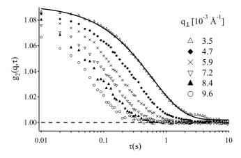
FIG. 2. Autocorrelation functions for a nematic sample with  $\phi_g = 6.7\%$  at different scattering vectors  $q_{\perp}$ . The solid line is the fit with a stretched exponential (the stretching exponent is about 0.6 for all the curves).
