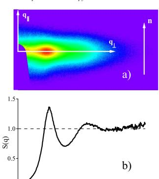
FIG. 1. a) SAXS pattern of an aligned nematic sample with  $\phi_g = 6.7\%$  at 228 K. The arrow indicates the direction of the nematic director  $\vec{n}$ . b) Structure factor along the  $q_{\perp}$  direction calculated from the SAXS data in a).
