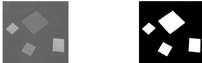
Fig. 11. Original image is first filtered using a Gaussian 3x3 filter and then thresholded (threshold value = 110). At last, small regions are deleted.
