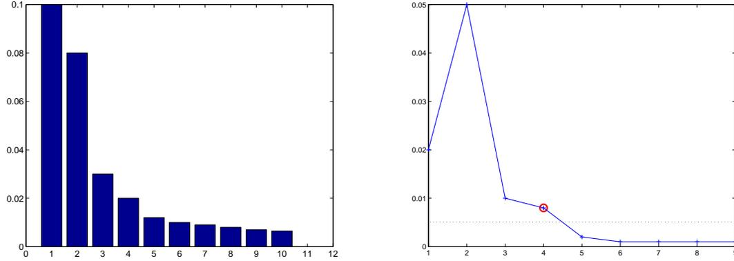
Figure 3: Estimation of the intrinsic dimension  $d_i$  using the scree-test of Cattell: plot of ordered eigenvalues of  $\Sigma_i$  (left) and differences between consecutive eigenvalues (right).
