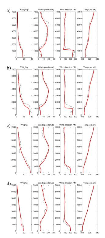
**Fig. 7.** Vapour mixing ratio (g/kg), wind speed (m/s) wind direction (deg) and potential temperature (K) derived from dropsonde measurements (red lines) and the MESONH simulation (black lines) at  $12^{\circ}$  N (**a**, DS1), at  $10^{\circ}$  N (**b**, DS2), at  $8^{\circ}$  N (**c**, DS3) and at  $6^{\circ}$  N (**d**, DS4) on 13 June.
