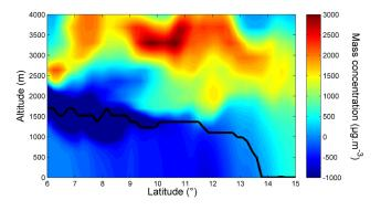
**Fig. 12.** Difference of dust mass concentration between the simulation without sedimentation (NOSED) and the simulation including sedimentation (SED; see text for more details) at 12:00 UTC on 13 June. Negative mass concentrations correspond to sedimented particles. The black line illustrates the top of the monsoon flux.
