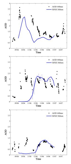
**Fig. 4.** Aerosol Optical Depth measured from 9 to 16 June 2006 over three Aeronet stations: Maine Soroa, Niger (**a**), Banizoumbou, Niger (**b**) and Djougou, Benin (**c**).
