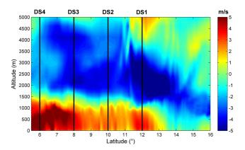
**Fig. 6.** Vertical cross section (along the ATR-42 flight track at  $2.00^{\circ}$  E) of the meridional component of the simulated wind (m/s). The black lines indicate the location of the dropsondes released by the F-F20 along the transect. The numbers refer to the dropsonde numbers as they appear in Fig. 7.
