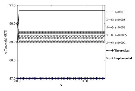
Fig. 7. Ratio between tangential stress and tangential displacement (case d).
