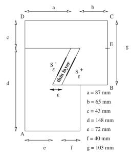
Fig. 4. The dovetail assembly.
