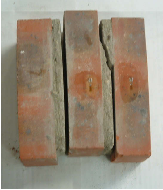
Fig. 7. Rupture mode in specimen.
