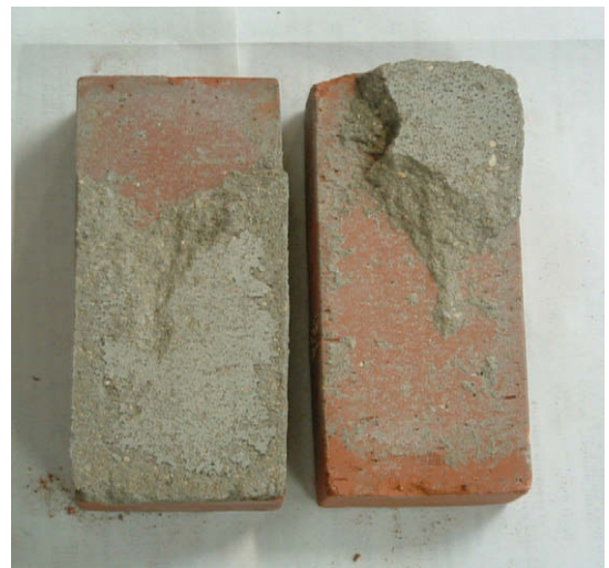
Fig. 6. Rupture mode in a specimen.
