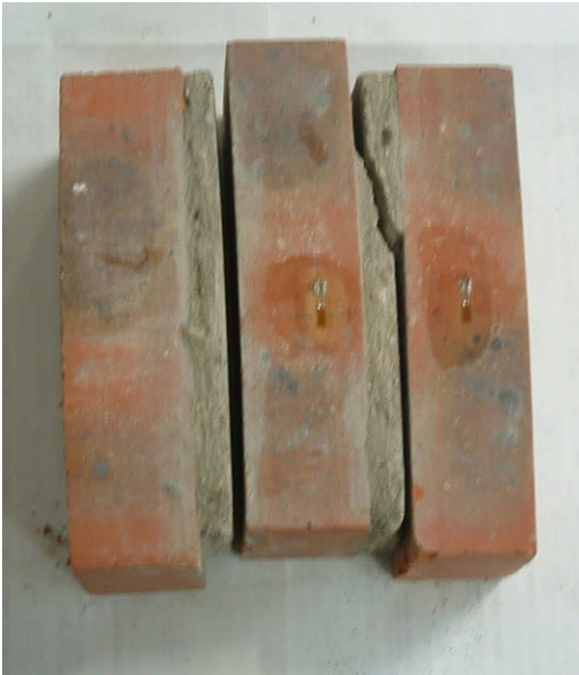
Fig. 7. Rupture mode in specimen.
