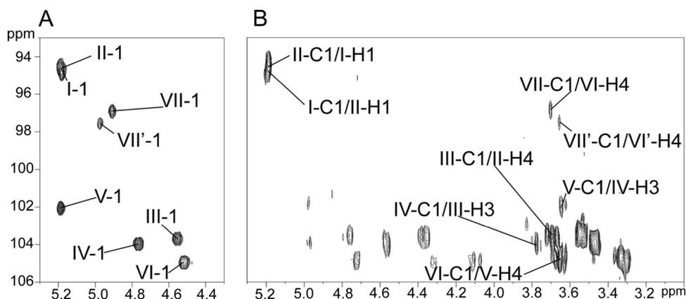
FIGURE 6. **Sequence analysis of OS-II by NMR.** Expanded areas of two-dimensional  $^1\text{H}$ - $^{13}\text{C}$  HSQC spectrum (A) and  $^1\text{H}$ - $^{13}\text{C}$  HMBC spectrum of OS-II fraction (B) are shown.
