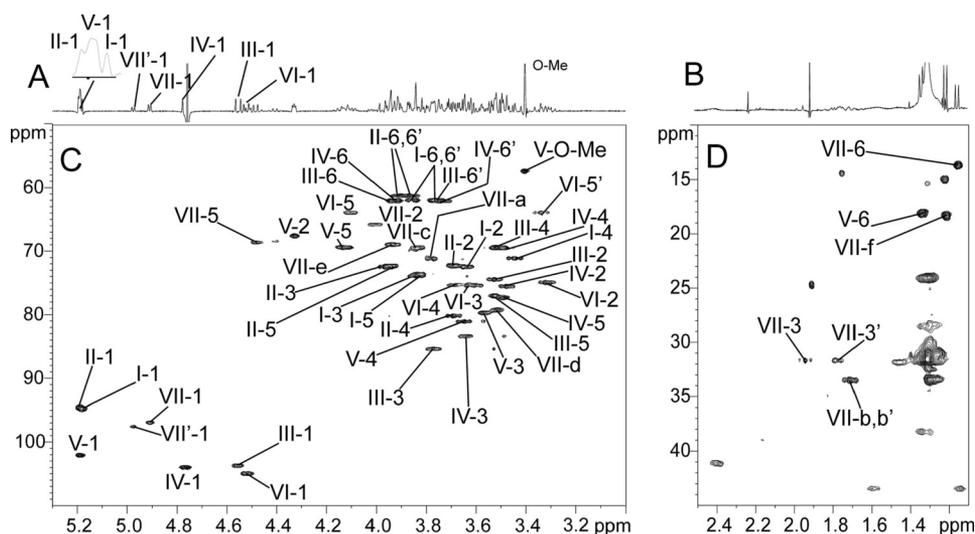
FIGURE 5.  $^1H$ - $^{13}C$  NMR analysis of OS-II fraction. Details of the anomer and bulk regions of the  $^1H$  NMR spectrum (A) and the  $^1H$ - $^{13}C$  HSQC NMR spectrum of OS-II (C) are shown. Details of the methyl and methylene resonances containing regions of the  $^1H$  NMR spectrum (B) and of  $^1H$ - $^{13}C$  HSQC NMR spectrum of OS-II (D) are shown.
