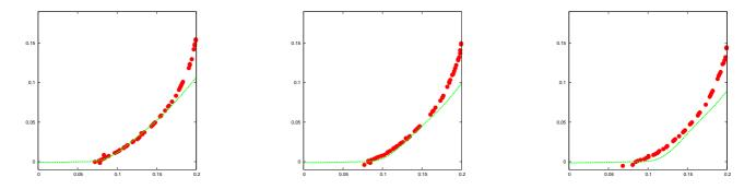
It is clear that during the first stage of penetration (up to  $t \approx 6ms$ ) the present model accurately predicts the size of the wetted surface and its expansion. In particular the fact that the wetted surface becomes almost flat is well reproduced. The following figures show the time variation of the radius of the wetted surface and its time derivative. In the right figure both rigid case  $(da/dt = \frac{3RV}{2a})$  and present elastic case are drawn
