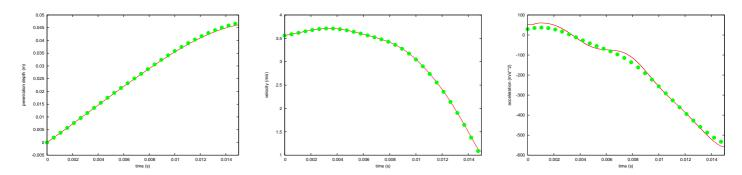
The computations provide the deformed shapes at some discrete instants (roughly at the first six milliseconds, those are plotted below (solid lines) and compared to measured data (dots)
