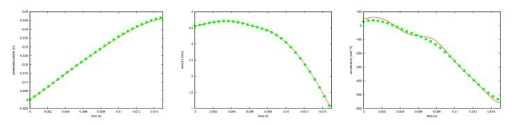
The computations provide the deformed shapes at some discrete instants (roughly at the first six milliseconds, those are plotted below (solid lines) and compared to measured data (dots)
