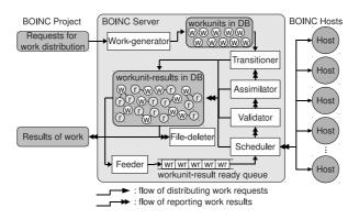
Fig. 1. Internal structures of BOINC server
