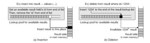
Fig. 5. Data insertion and deletion examples in RT-BOINC
