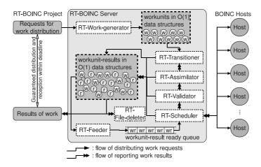
Fig. 3. Internal structures of RT-BOINC server
