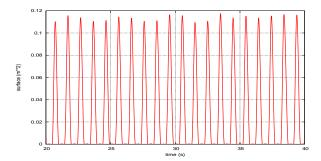
It is worth noticing that the positive and negative maxima of the force are of the same magnitude. This was also revealed by Barrholm (2001). These plots also show that the repeatability of each impact of standing wave crest is reasonable consistently with the repeatability of the measured wave kinematics. In order to check this point, the force is plotted in term of the wetted surface (figure below, on the left).
