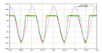
When the flate plate is hitted, the wave gauges saturate at a threshold which corresponds to the airgap h. What is most noticeable is the larger slope of the ascending wave. This means that the local vertical velocity increases due to presence of the flat plate. This vertical velocity is calculated by a time differentiation of the wave elevation. This leads to a very irregular signal and a smoothing is necessary. The figure below shows a time sequence of the velocity variation.
