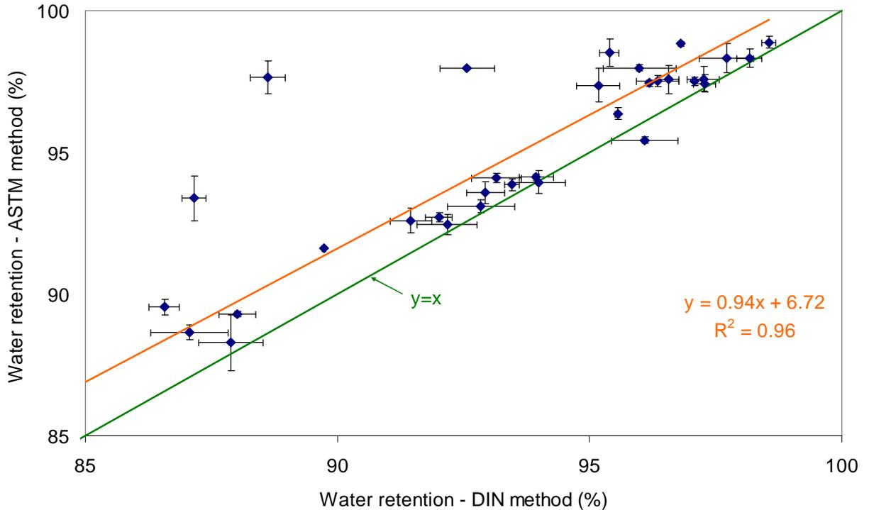
**Fig. 3.** Comparison between the DIN and the ASTM method.
