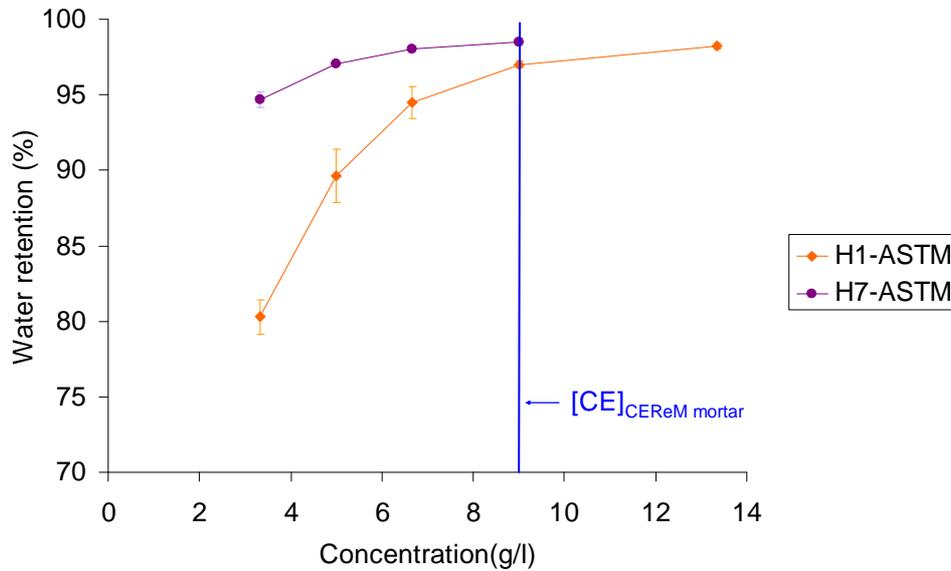
**Fig. 8.** Influence of HEC concentration on water retention.
