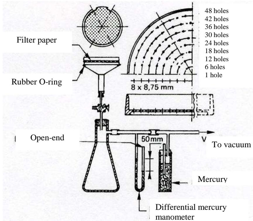
**Fig. 2.** Experimental device to measure water retention with standard ASTM C91.
