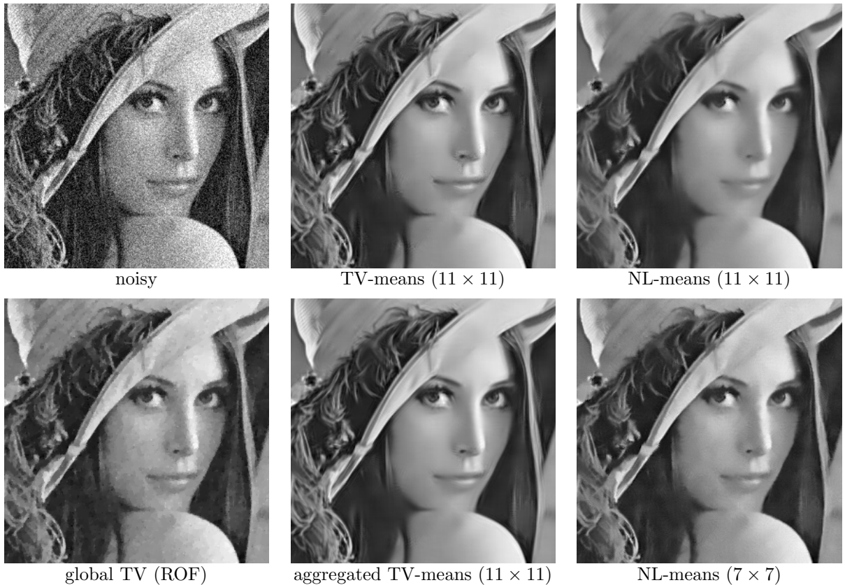
Figure 8: Denoising of Lena image (detail). As in Figure 7, global TV-denoising simultaneously leaves noise (and staircasing) on the smooth parts and erases some texture (hat, feathers). The NL-means method performs better, but either leaves noticeable noise ( 7 \times 7 patches), or introduces too much blur ( 11 \times 11 patches). A more balanced treatment of edges, flat areas and textures is obtained with aggregated TV-means, yielding a better global impression and a more precise recovery of textures (see, e.g., the feathers and the thin stripes of the hat).
