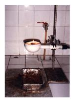
**Fig 2.** Experimental device used in the firebrands tests
