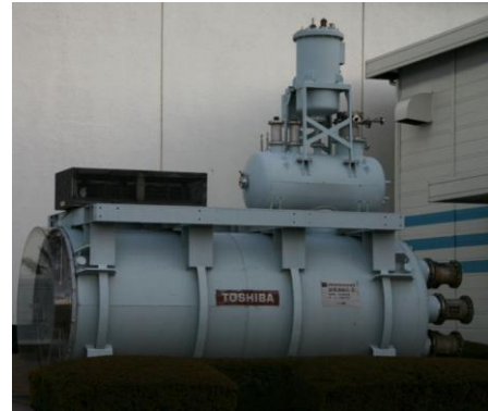
Fig. 1. A MHD thruster from the experimental Japanese ship Yamato 1 at the Ship Science Museum in Odaiba, Tokyo.
