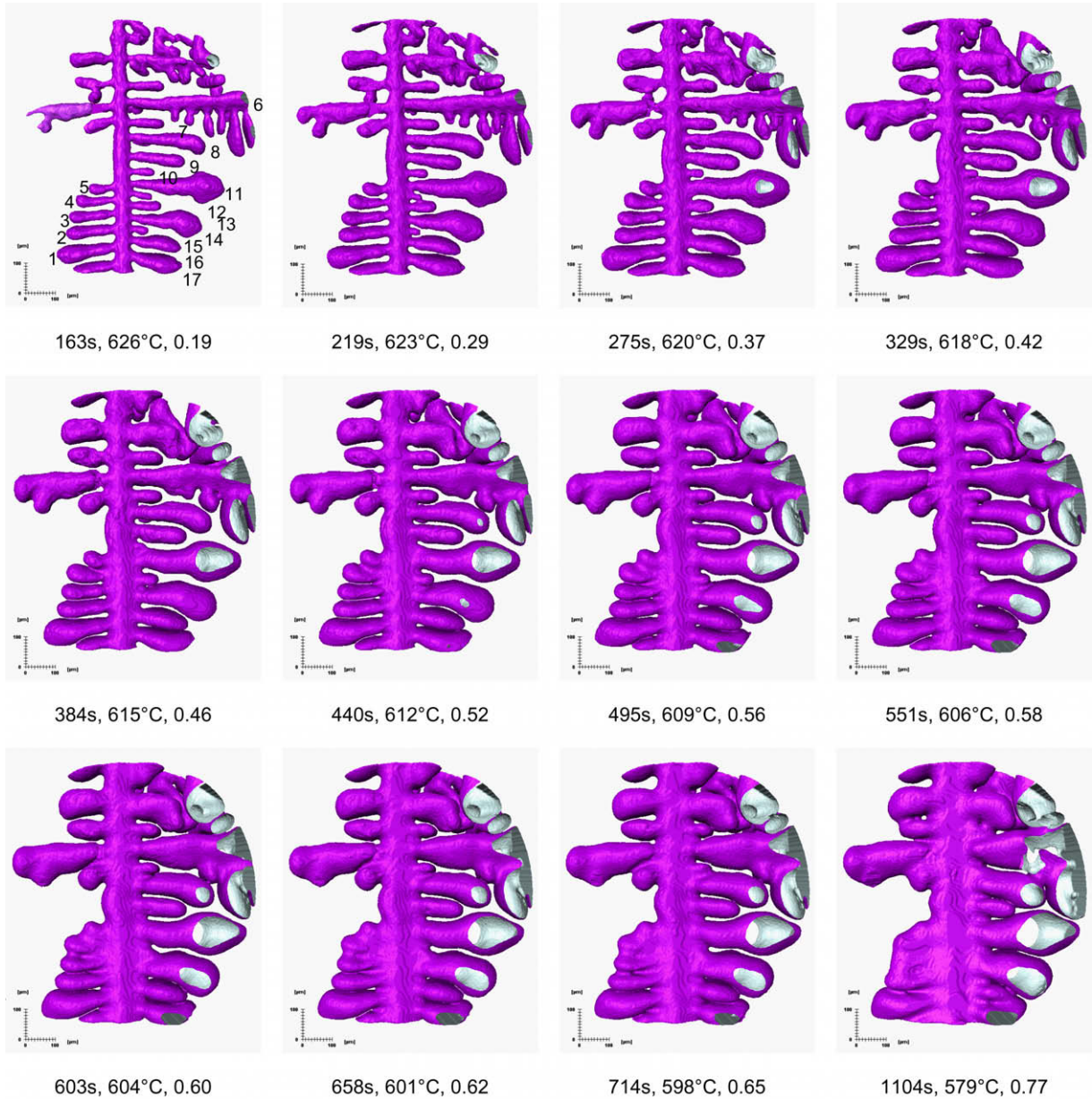
Fig. 6. Three-dimensional observation of the evolution of a dendrite with solidification time.
