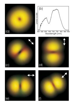
FIG. 2. (Color) (a) Image of the radially polarized polychromatic beam. (b) Chromatic spectrum of the optical source (linear scale). [(c)-(f)] Image of the radially polarized beam after passing through an analyzer whose axis directions are indicated by white arrows.
