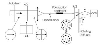
FIG. 1. Scheme of the experimental setup of generation and imaging of the polychromatic radially polarized beam.
