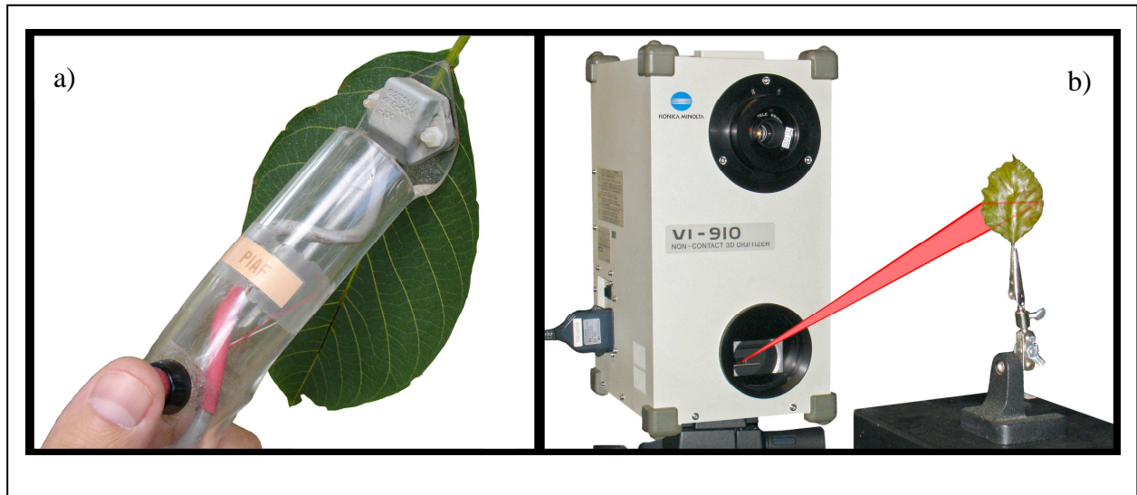
521 Fig. 1. Illustration of two digitizing methods: a) Leaf digitizing in a tree with a hand-held 522 electromagnetic digitizer 3Space Fastrack Polhemus; the pointer is set parallel to the midrib 523 and the mean plane of the lamina and points the junction between petiole and lamina. b) Leaf 524 digitizing with a non-contact laser scan digitizer Konica Vi-910 on detached leaves. The light 525 red triangle mimics the emitted laser plane.
