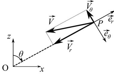
Figure 1: Definition of velocity components in a vertical plane ( $x - z$ )
