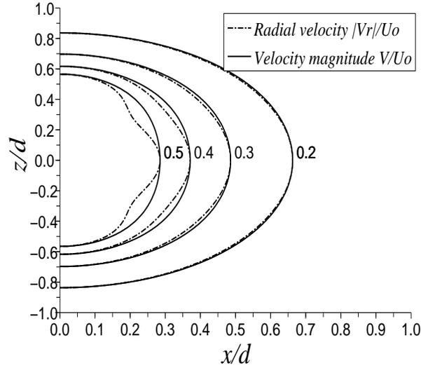
Figure 3: Iso-velocity lines in  $x - z$  plane
