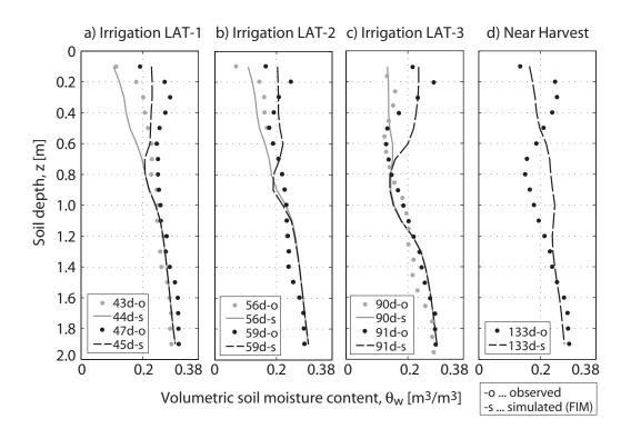
Figure 7: Simulated and observed soil moisture profiles at  $x = 20 m / x_{inf} = 32.5 m$  for various times of the 1999 growing season at Lavalette
