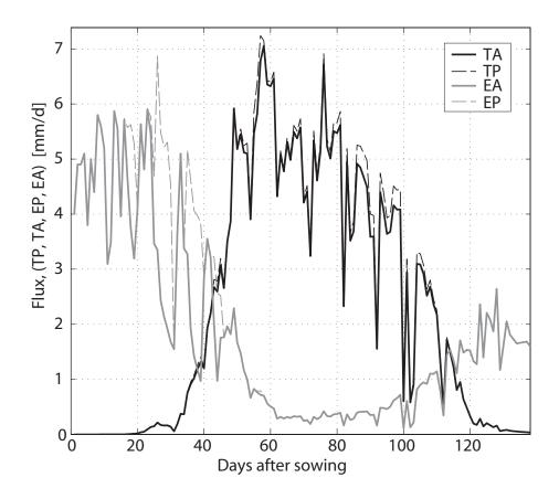
Figure 9: Simulated components of evapotranspiration at  $x_{inf} = 32.5 m$  during the entire growing season of the Lavalette run: potential transpiration TP, actual transpiration TA, potential evaporation EP and actual evaporation EA
