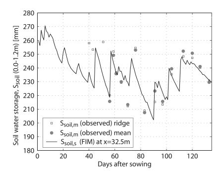
Figure 6: Observed and simulated soil water storage at the upstream section,  $x_{inf} = 32.5 m$ , during the entire 1999 growing season of corn at Lavalette
