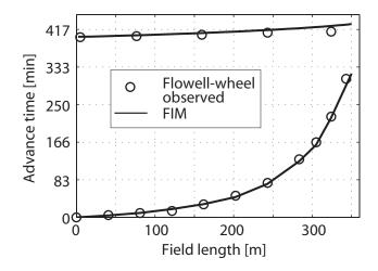
Figure 5: Observed and simulated advance and recession times for the Flowell-wheel run
