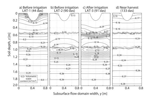
Figure 8: Simulated soil moisture distribution at  $x_{inf} = 32.5 m$  for various times of the 1999 growing season at Lavalette
