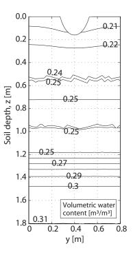
Figure 2: Initial soil moisture distribution, as simulated for the day of sowing of the Lavalette run
