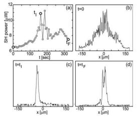
Fig. 10. Experimental results performed with a 40 kV/cm applied field, a 760  $\mu$ W infrared input power, and a temperature of 5 °C. (a) SH output power evolution and (b)–(d) SH output mode profile along the *c* axis taken at three different times, as marked in graph (a).
