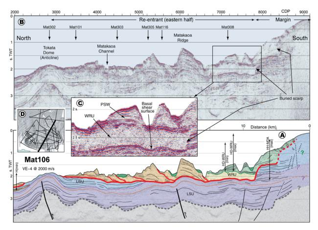
**Figure 6.** MCS reflection profile Mat106 across the Matakaoa Reentrant. (a) Interpreted profile and (b) uninterpreted processed data. (c) Enlargement on the weakly reflective unit, showing the strong negative reflector indicating the basal shear surface, and the overlying Postavalanche Sedimentary Wedge. (d) Location of profile. See Figure 5 for full caption and color legend and Figure 2 for location of seismic profiles.
