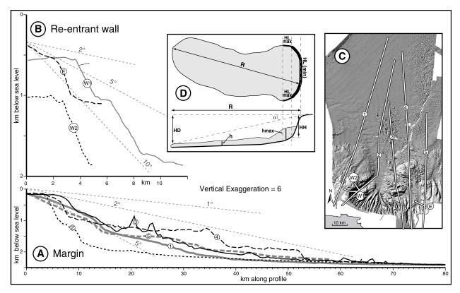
**Figure 4.** Bathymetric profiles across the margin and the reentrant. (a) The Matakaoa Margin includes the continental slope on either side of the reentrant (profiles 1 and 5, i.e., along the nonfailed parts of the margin) and within the reentrant (profiles 2, 3, and 4). (b) Western and eastern reentrant walls. (c) Map showing profile locations. (d) Sketch of the various morphometric parameters used in text and Tables 2 and 3.
