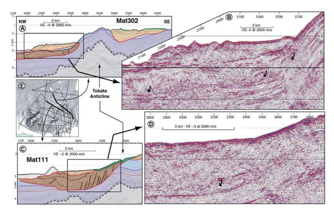
**Figure 8.** Parts of MCS reflection profiles (a) Mat302 and (c) Mat111 over the NW flank of the Tokata Anticline. Enlargements of uninterpreted seismic reflection profiles (b) Mat302 and (d) Mat111 showing the extension of the Raukumara Slump to the south and the collapsed flank of the anticline. (e) Inset shows the location of seismic profiles. See Figure 5 for full caption and color legend and Figure 2 for location of seismic profiles.
