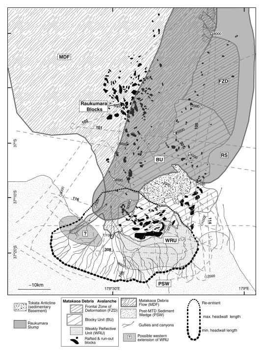
**Figure 11.** Present-day extents of the mass transport deposits of the Matakaoa Submarine Instability Complex (MSIC), as identified along the Matakaoa Margin and in the Raukumara Basin. Grey dash lines indicate seismic reflection profiles (see Figure 2).
