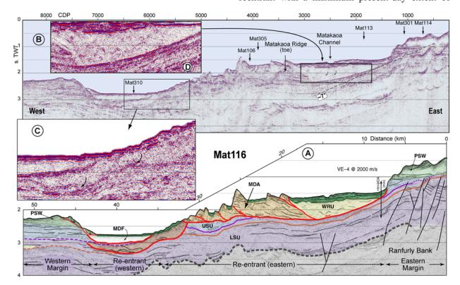
**Figure 7.** MCS reflection profile Mat116 across the Matakaoa Reentrant. (a) Interpreted profile and (b) uninterpreted processed data. (c) Enlargement on the failed western flank of the Tokata Anticline, and erosional basal surface of the MDF. (d) Enlargement on WRU showing back-tilted reflectors. Curved arrows indicate interpreted back-tilted blocks. See Figure 5 for full caption and color legend and Figure 2 for location of seismic profiles.
