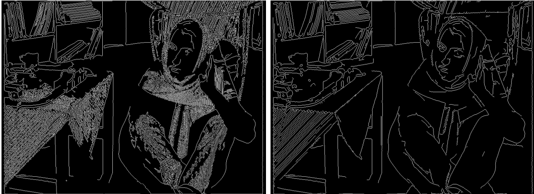
Figure 5: Canny's edge detector applied on the original Barbara image, and Canny's edge detector applied on the cartoon image obtained by the proposed algorithm in Figure 3. Edges caused by the textures are eliminated.
