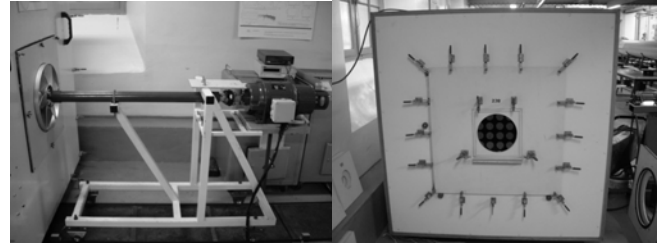
Figure 2: ISO 5801 air test bench, Dynfluid-LEMFI / Arts et Métiers ParisTech. The dimensions are 1.3 x 1.3 x 1.8 m.
