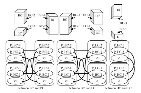
Fig. 8. Layout modeling with ports and connections.
