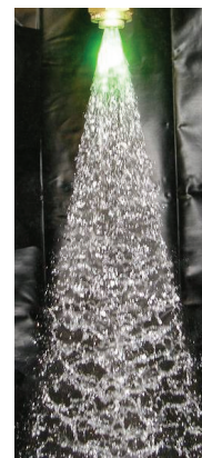
FIG. 1: sketch of the nozzle orifice and photograph of the experimental set-up (Lechler Nozzle ref. 665-042, 8 bars)
