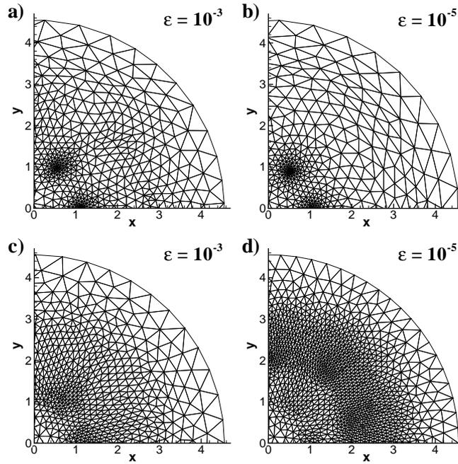
Figure 7:  $\Omega = 2.5$  Mesh evolution during the computation for experiment 2 (see Fig. 6). Refined meshes corresponding to thresholds  $\varepsilon = 10^{-3}$  and  $\varepsilon = 10^{-5}$ . Adaptive mesh strategy using  $\chi = |u|$  (a and b) and  $\chi = [u_r, u_i]$  (c and d).
