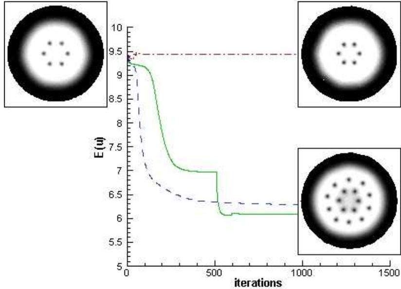
Figure 6: Computation for  $g = 500$ ,  $\Omega = 2.5$  and combined harmonic-plus-quartic trapping potential. Computations start from the converged state obtained for  $\Omega = 2$ . Energy evolution for constant mesh ( $M = 400$ , dashed line) and different adaptive mesh computations:  $\chi = |u|$  (dash-dot line) and  $\chi = [u_r, u_i]$  (solid line). Density contours ( $|u|$ ) for initial and converged solution (low density in black).
