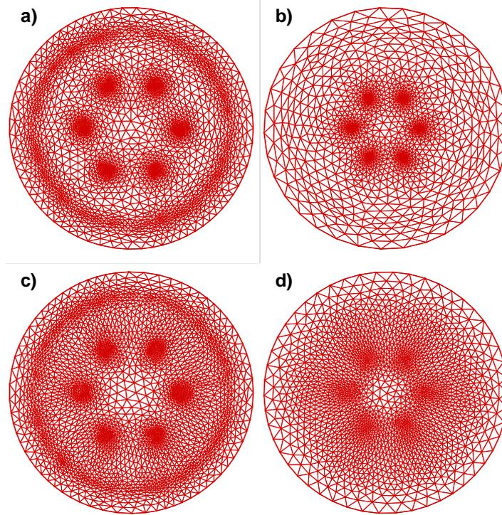
Figure 5: Mesh evolution during the computation for experiment 1 (see Fig. 3). First ( $\varepsilon = 10^{-2}$ ) and final ( $\varepsilon = 10^{-5}$ ) refined meshes are represented for the adaptive mesh strategy using  $\chi = |u|$  (a and b) and  $\chi = [u_r, u_i]$  (c and d).
