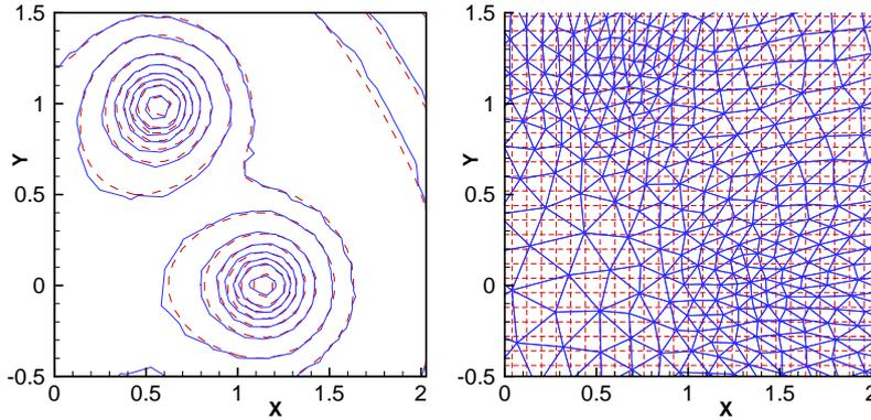
Figure 4: Computational case depicted in Fig. 3. Comparison between the results obtained with the finite element method for  $M = 200$  and mesh adaptivity using  $\chi = [u_r, u_i]$  and the 6th order finite difference method with a  $105 \times 105$  equally spaced grid. Details of the contours of the atomic density  $|u|$  and corresponding grids (dashed lines for the finite difference results).
