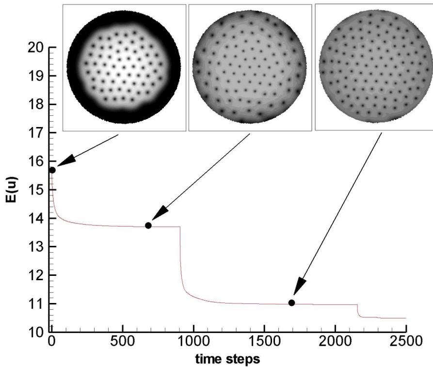
Figure 2: Illustration of the imaginary time evolution of the solution before reaching the converged state displayed in Fig. 1. Energy decrease and contours of atomic density  $\rho$  for intermediate states. Note the nucleation of new vortices and their rearrangement in a more and more regular Abrikosov lattice. The jumps in the energy evolution correspond to mesh refinement.
