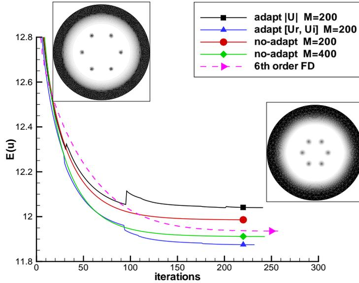
Figure 3: Computation for  $g = 500, \Omega = 2$  and combined harmonic-plus-quartic trapping potential. Initial condition with 6 vortices artificially placed at  $0.5 \cdot R_{TF}^\Omega$ . Energy evolution for constant mesh and different adaptive mesh computations; the result obtained with a 6th order finite difference method is also plotted for comparison. Density contours ( $|u|$ ) for initial and converged solution (low density in black).
