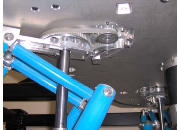
Fig. 4. Actuation system of each leg.
