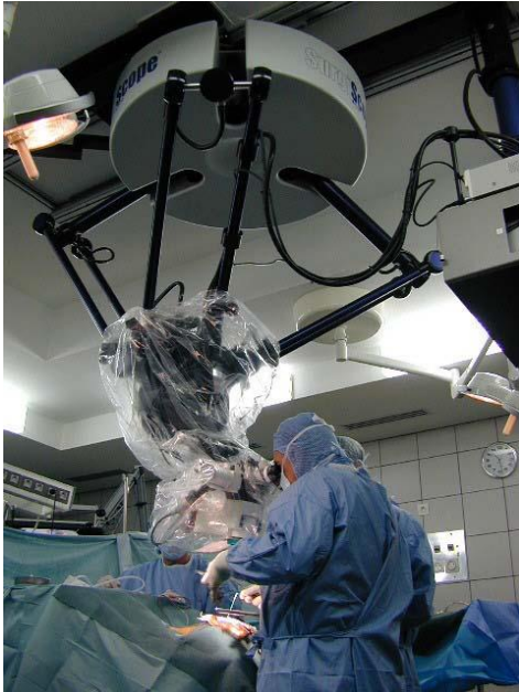
FIG. 1. SURGISCOPE ® , A ROBOTIZED NAVIGATION TOOL-HOLDER DESIGNED FOR NEUROSURGERY DEVELOPED BY THE ISIS COMPANY.
