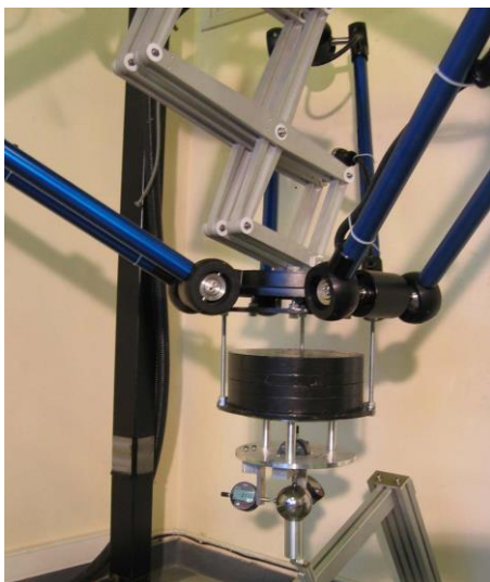
FIG. 11. MEASURING OF THE POSITIONING ERRORS FOR GIVEN STRAIGHT LINE TRAJECTORY.
