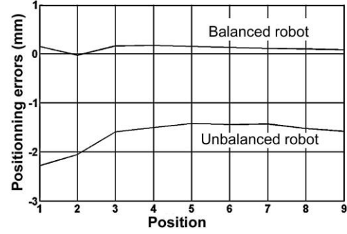
FIG. 12. RELATIVE POSITIONING ERRORS WITH RESPECT TO Z AXIS FOR UNBALANCED AND BALANCED ROBOTS.
