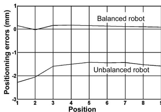
Fig. 17. Relative positioning errors with respect to z axis for unbalanced and balanced robots.
