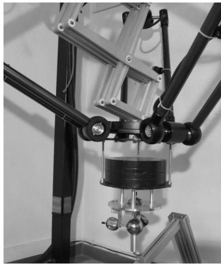
Fig. 16. Measuring of the positioning errors for given straight line trajectory.
