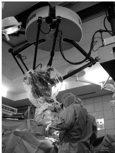
Fig. 1. A Delta robot used in the SurgiScope ® , a robotized navigation tool-holder designed for neurosurgery and developed by the ISIS 2 company.
