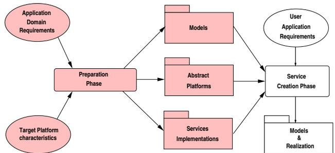
**Fig. 2** Development flow to embed a humanoid robot in an application providing a Collaborative Working Environment
