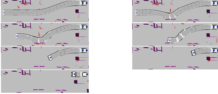
Fig. 3 A backward trajectory computed and executed by the mobile robot Hilare 2 towing a trailer. Grey dots are obstacles detected by a laser range finder mounted on the trailer. An unexpected box lies on the trajectory planned by the robot. The robot deforms the trajectory while moving and reach the goal.
