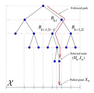
Figure 1: Illustration of the node selection procedure in round n. The tree represents  $\mathcal{T}_n$ . In the illustration,  $B_{h+1,2i-1}(n-1) > B_{h+1,2i}(n-1)$ , therefore, the selected path included the node (h+1,2i-1) rather than the node (h+1,2i).
