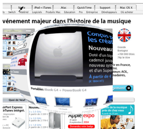
Figure 10. Transparent appearance of a view of a page while the pointer hovers over one of the links of a web page (without displaying the plan)
