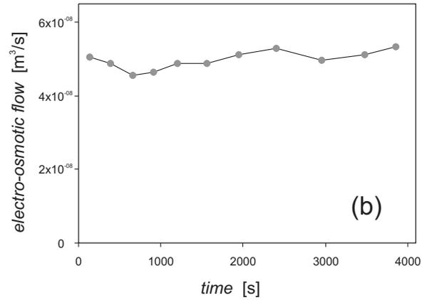
Figure 2: Experimental results with a 26mm thick sample submitted to a 10V electrical potential difference: (a) oil bubble displacement as a function of time - (b) electro-osmotic flowrate through the sample as a function of time.
