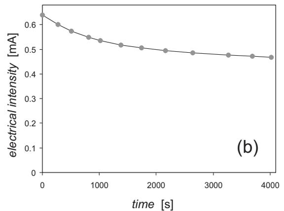
Figure 3: Experimental results with a 26mm thick sample submitted to a 10V electrical potential difference: (a) electrical potential difference between both sides of the sample - (b) ionic current intensity through the sample.
