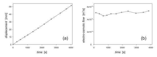
Figure 2: Experimental results with a 26mm thick sample submitted to a 10V electrical potential difference: (a) oil bubble displacement as a function of time - (b) electro-osmotic flowrate through the sample as a function of time.
