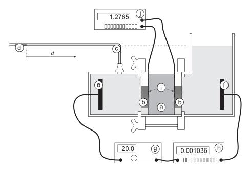
Figure 1: Experimental device for the determination of the electro-osmotic permeability of Agar-Agar gel sample
