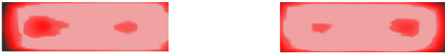
Fig. 2. Current displacement in the conductor cross section of the two turn side of the test inductor. Plot obtained by HFSS-simulation of the test-inductor, current density in logarithmic scale increasing to darker colors (see figure 3). The slightly higher current in the very inside of the metal is due to small simulation inaccuracies.
