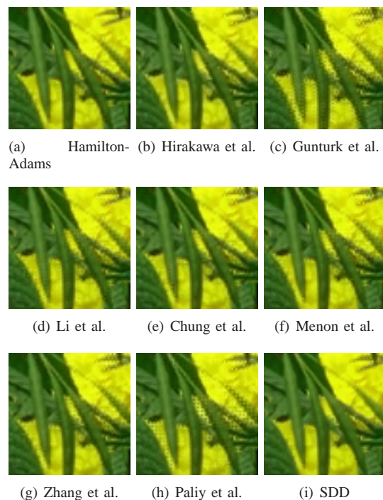
Figure 10. Zipper effect on IMAX images. Most methods present a strong zipper effect on color edges that makes the demosaicked image not a reasonable solution to the demosaicking problem. Only the SDD algorithm and Hamilton-Adams are able to give a reasonable solution.
