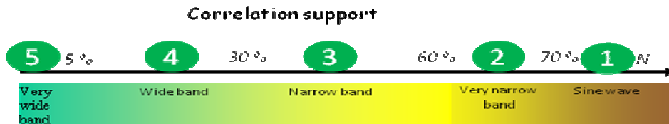
Figure 3. Correlation support and size of the signal spectral band.
