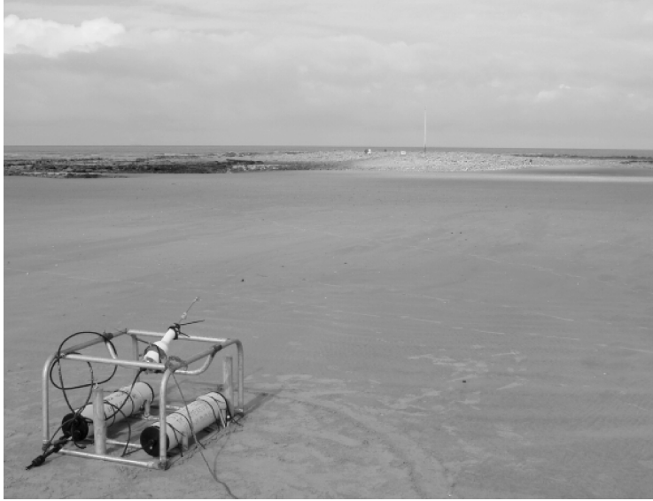
Fig. 2. A photography of the ADV measuring device and its support, in the intertidal zone, before being submerged by the tide.
