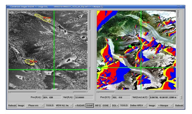
**Figure 7:** display of two stacks of data (radar geometry at left and georeferenced at right) linked thanks to the processed LUT.
