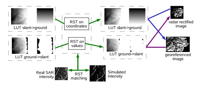
**Figure 3:** Final RST matching to improve the LUT accuracy. The final transformation is applied on the images of the geocoding LUT and on the values of the radar-coding LUT.
