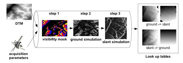
Figure 1: processing chain to build the LUT allowing to radar rectify georeferenced data and to geocode SAR image.
