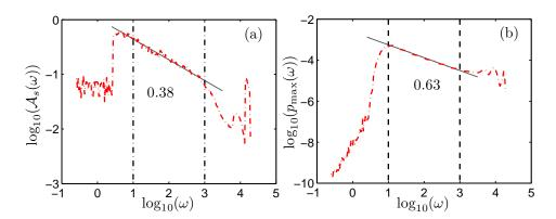
Fig. 5: The skeleton of the joint pdf. (a)  $\mathcal{A}_{\rm s}(\omega)$  in log-log plot. A power law behaviour is observed in the inertial subrange with scaling exponent 0.38, which is close to the Kolmogorov value 1/3. (b)  $p_{\rm max}(\omega)$  in log-log plot. A power law behaviour is observed in the inertial subrange with scaling exponent 0.63. The vertical lines show the corresponding inertial subrange  $10 < \omega < 1000\,{\rm Hz}$ .
