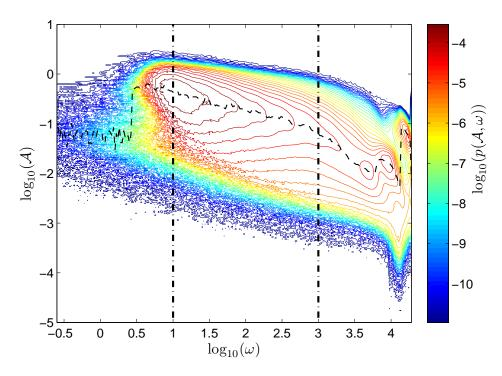
Fig. 4: Representation of the joint pdf  $p(\omega, \mathcal{A})$  (in log scale) of turbulent fluctuations in an amplitude-frequency space. The scaling range  $10 < \omega < 1000\,\mathrm{Hz}$  for frequencies is shown as vertical dotted lines. The dashed line shows the skeleton  $\mathcal{A}_\mathrm{s}(\omega)$  of the joint pdf, which is the amplitude for which the conditional pdf  $p(\mathcal{A}|\omega)$  is maximum.
