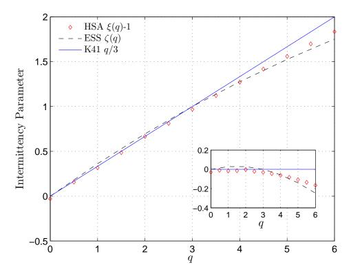
Fig. 8: Comparison of the scaling exponents  $\xi(q) - 1$  (diamond) with the classical  $\zeta(q)$  obtained from structure functions analysis with the ESS method (dash-dotted line) and K41 q/3 (solid line). The insert shows the departure from the K41 law.
