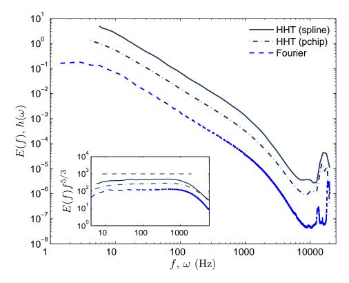
Fig. 1: Comparison of the Hilbert marginal energy spectrum (solid line) and Fourier spectrum (dashed line, vertically shifted). The slope of the reference line is -5/3. Both the second order Hilbert and Fourier spectra indicate the same inertial subrange, 10 < f (or  $\omega$ ) < 1000 Hz. The insert shows the compensated spectra. The HHT spectra estimated using two different algorithms are shown for comparison, indicating a stability of the spectrum with respect to the algorithm used.
