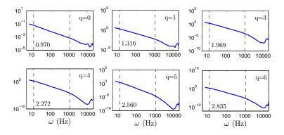
Fig. 7: Representation of  $\mathcal{L}_q(\omega)$ , Hilbert spectral analysis of velocity intermittency, using different orders of moments (0, 1, 3, 4, 5 and 6). Power laws are observed on the range  $10 < \omega < 1000\,\mathrm{Hz}$  for all spectra. The value of the scaling exponent  $\xi(q)$  is shown in each figure.
