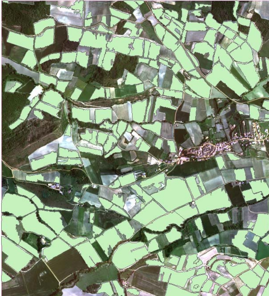
Figure 4.12. Results of the segmentation on the red channel of the INTA image, Limoux test-site (France)
