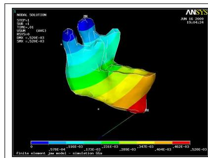
Figure 1. Dynamic jaw simulation for opening in ANSYS with displacement field coloring.
